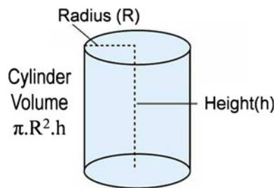
**Fig. 1** Cylinder volume
